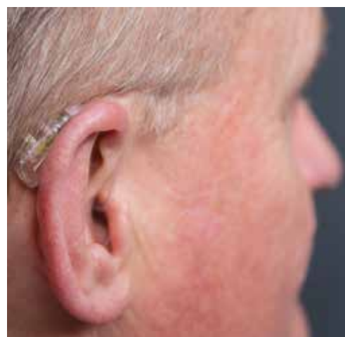
An antistuttering device developed at East Carolina University is now also being marketed and distributed to people with Parkinson's disease to assist them with speech. The SpeechEasy, marketed by Janus Development Group, is a portable device that fits in or behind the ear and can help people who stutter to speak more fluently. Studies have shown that the use of an auditory delay and/or a change in pitch can help increase the intelligibility of speech in those with Parkinson's disease as well.
