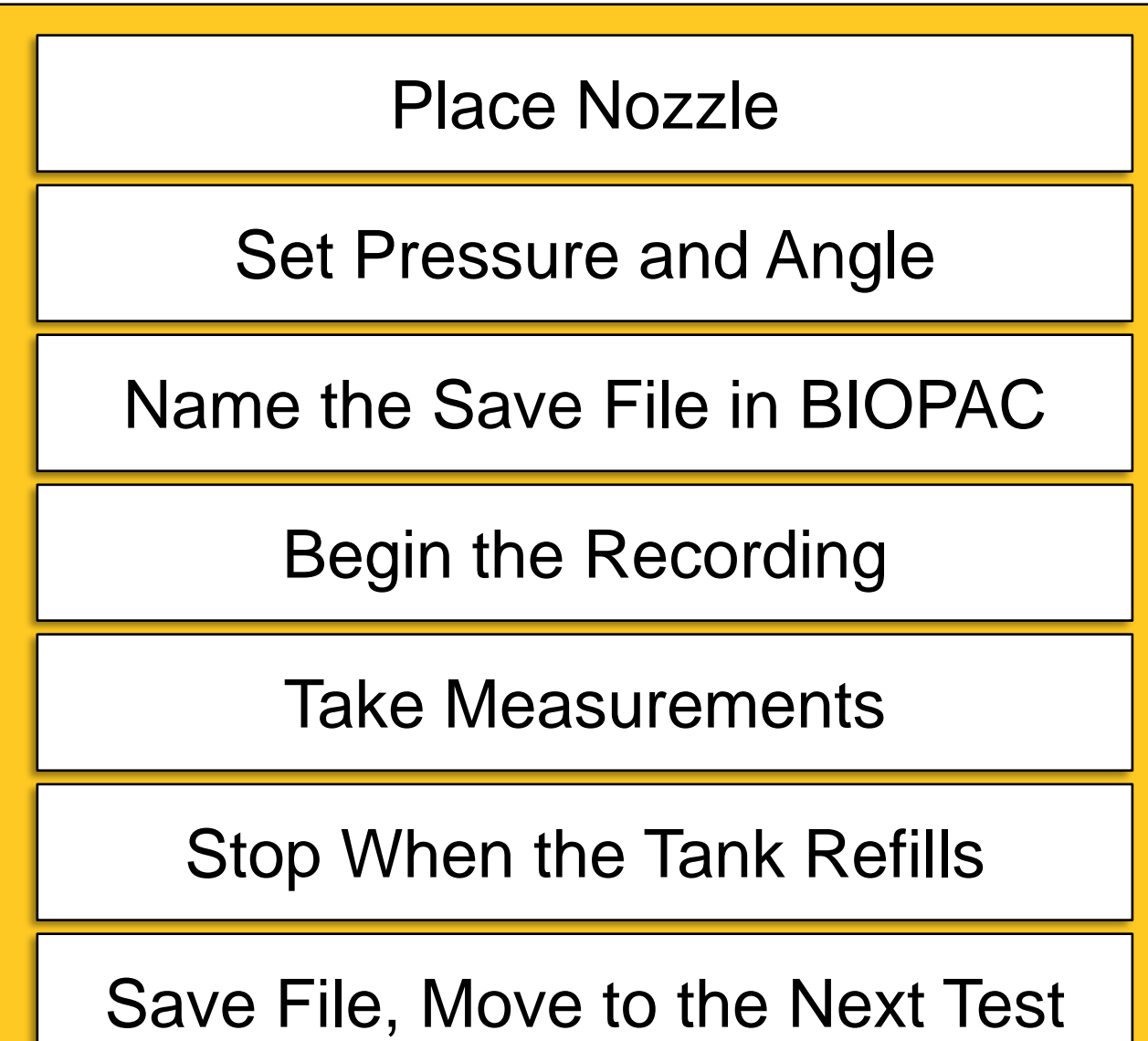
Figure 1. A flowchart detailing each process within the testing procedure.
